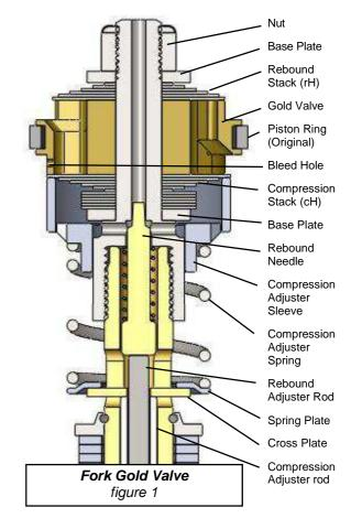
Check to see there are no burrs on the Gold Valve Piston and the piston faces are flat. If required, surface the piston on a piece of plate glass with 320 grit (very fine) sandpaper (the piston is surfaced from the factory but check it every time you disassemble the valving.) Put the original piston ring on the Gold Valve. Place the Gold Valve on the shaft with the piston face that uses the large diameter shim (6 ports) facing down against the Compression Stack.
